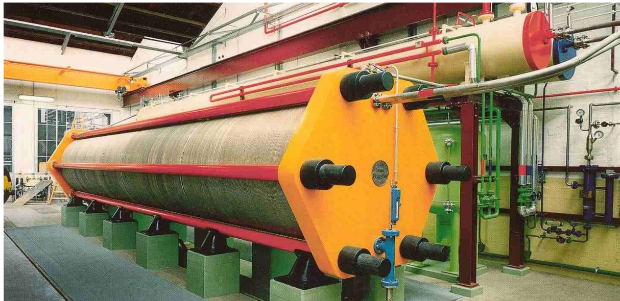
IHT, Lurgi, 3 MPa, capacity 760 Nm 3 h -1 , 5 MW
